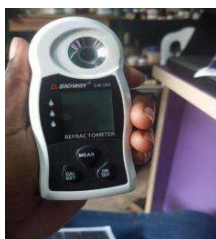
Figure 2.2.1: Handheld Digital Refractometer Used To Determine The Brix Value And Refractive Index Of The Extracted Citrus Peel Oil
