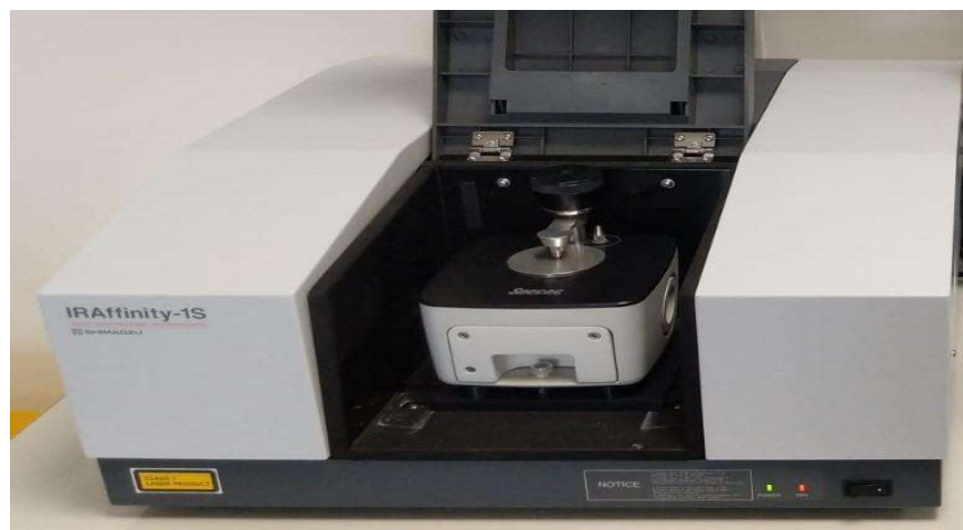
Figure 2.2.2: Fourier Transform Infrared (FTIR) Spectrophotometer Used For Functional-Group Analysis Of The Extracted Citrus Peel Oil
