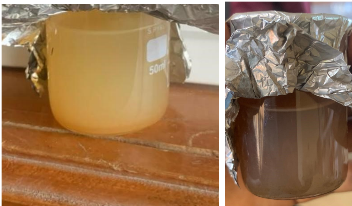
Figure 1: (a) \text{AgNO}_3 with ginger rhizome alkaloid-rich extract (b) Colourchange that indicated nanoparticles synthesis
